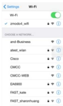
Select the WiFi network that your cameras will connect to, and connect to it. Return to the Funlux app once your mobile device is connected to the WiFi network.
